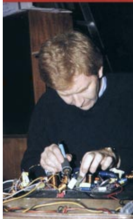
Alan Shaw fine tuning the Monitor 40's passive crossover.
